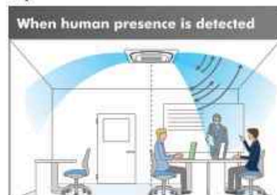
Optimal air direction by "Auto" Swing (narrow)
